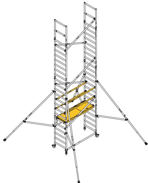
**12** Fit the trapdoor platform as shown. From the protected trapdoor position, fit horizontal braces as shown.
