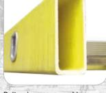
Pultrusion composed by fibreglass and resin stratified tissues
